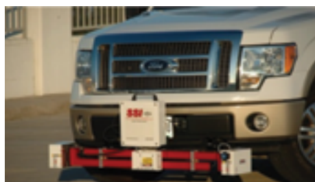
Figure 3.22. Noncontact lightweight profiler
