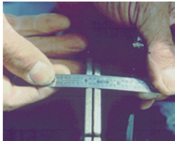
Figure 10.8. Ganged sawblades to provide desired cutting width
