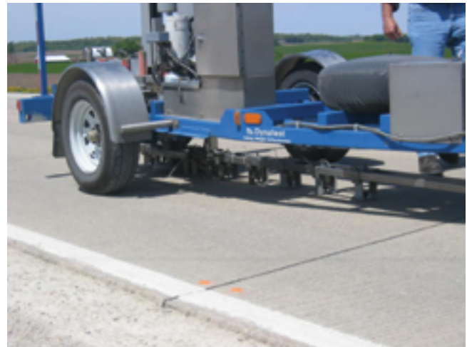
Figure 3.5. Example of FWD showing sensor bar
