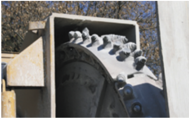
Figure 5.14. "V" shape milling head (top) and milling pattern (bottom) (Frentress and Harrington 2012)
