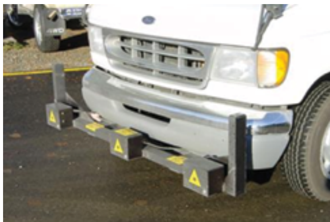
Figure 3.24. Example of high-speed profiler (photo courtesy of WSDOT)
