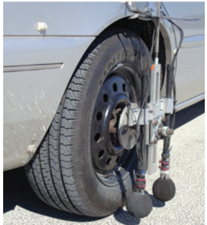
Figure 3.20. OBSI testing configuration (Rasmussen, Sohaney, and Wiegand 2011)
