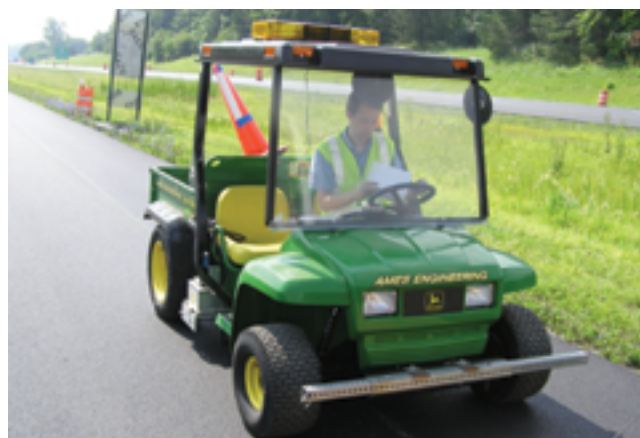
Figure 3.22. Noncontact lightweight profiler
