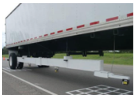
a. Rolling wheel deflectometer
