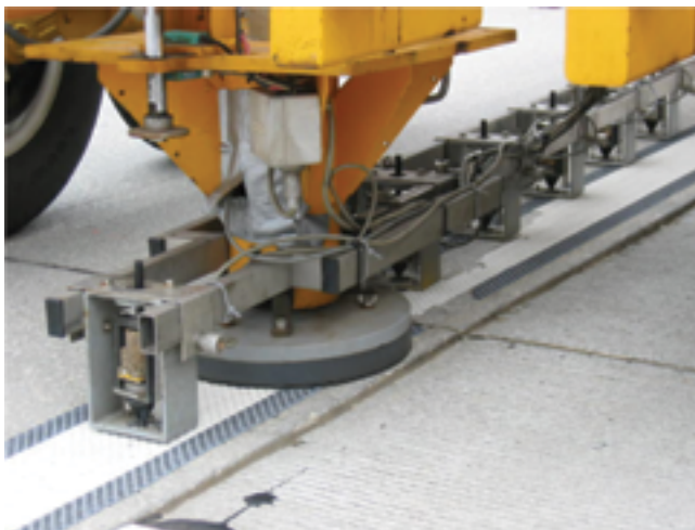
b. Measuring deflection load transfer
