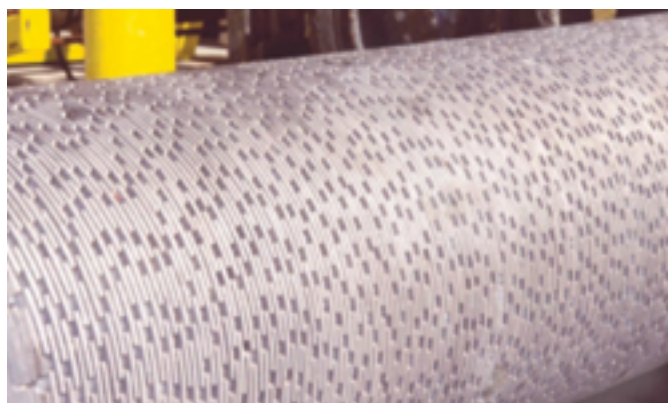
a. Conventional diamond grinding head
