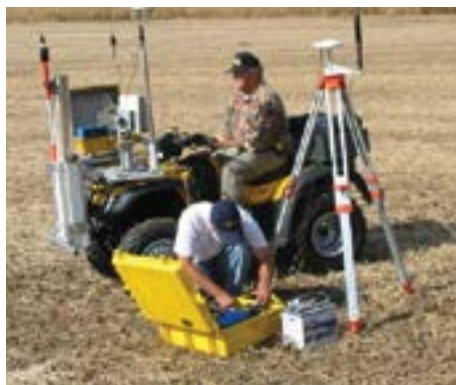
Figure 142. GPS base station mobile or fixed
