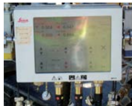
Figure 138. Computer controls on paving machine
