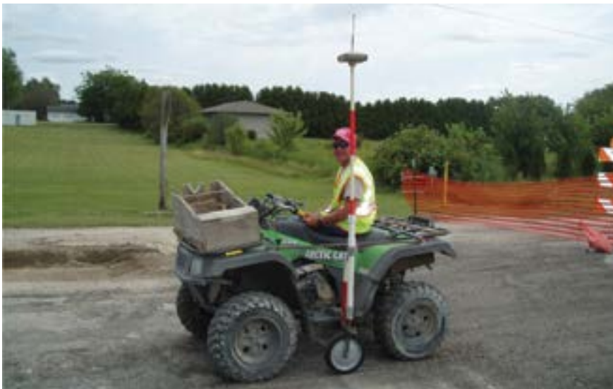
Figure 135. ATV with GPS and laser profile
