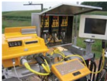
Figure 143. GPS paver control system
