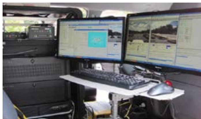
Figure 132. Mobile scanner onboard quality control operation area
