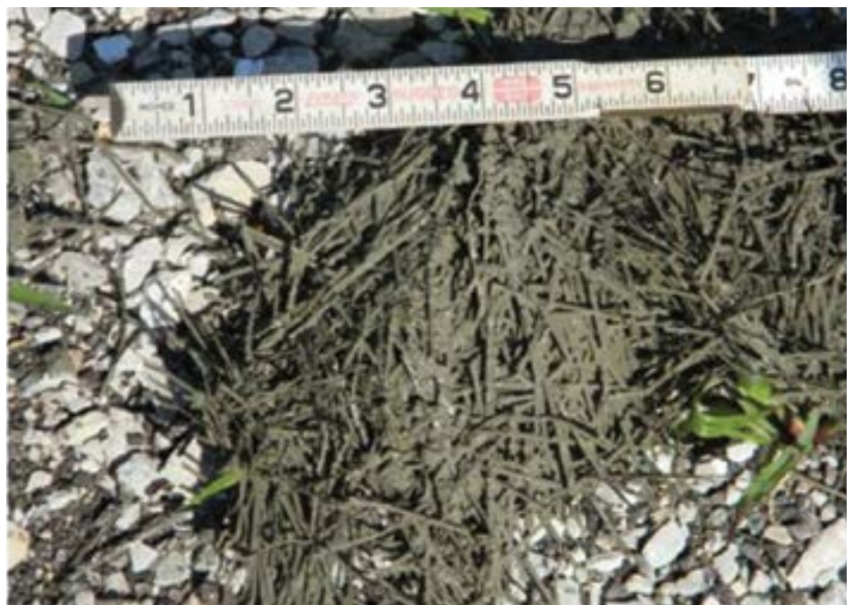
Figure 91. Synthetic fibers (1.5 in. to 2.25 in.)
