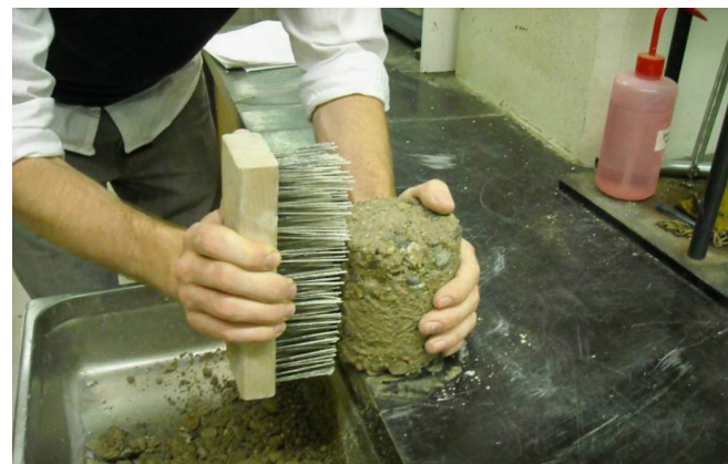
Figure 5.10. Brushing during freeze-thaw durability testing
