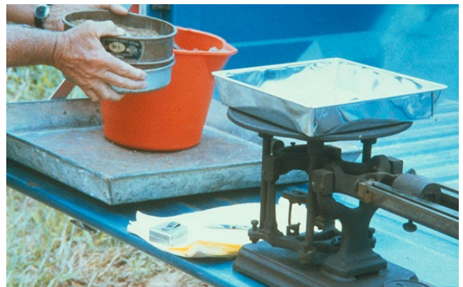
Figure 7.1. Gradation verification during construction
