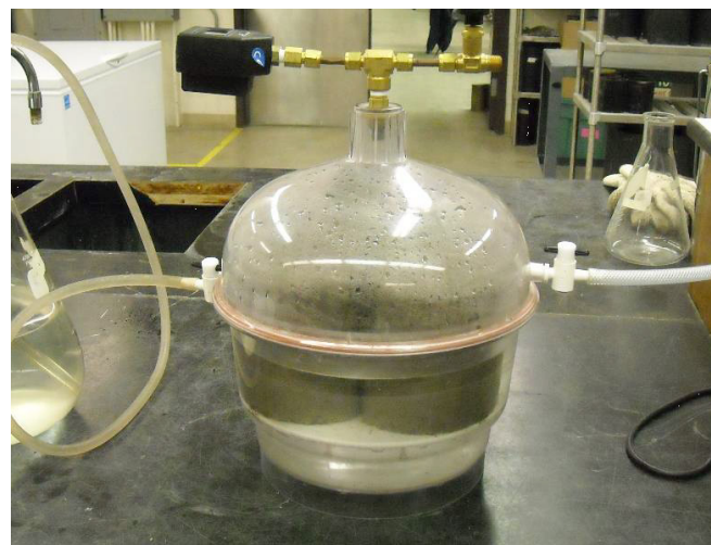
Figure 2.9. Specimens subjected to vacuum saturation testing
