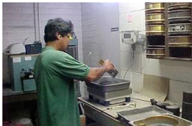
Figure 5.6. Gradation testing on existing materials
