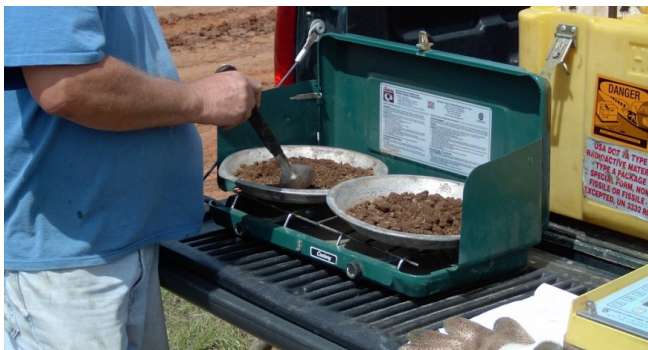
Figure 7.3. Drying an FDR sample by using a stove for moisture content verification
