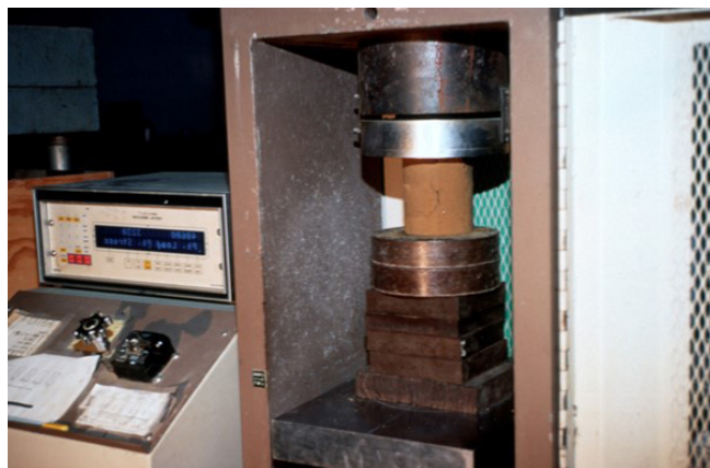
Figure 2.4. Unconfined compressive strength test being performed on an FDR with cement specimen
