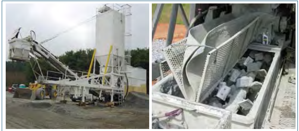
Figure 6-4. Continuous flow pugmill mixer (left) and close-up view of mixing chamber (right)
