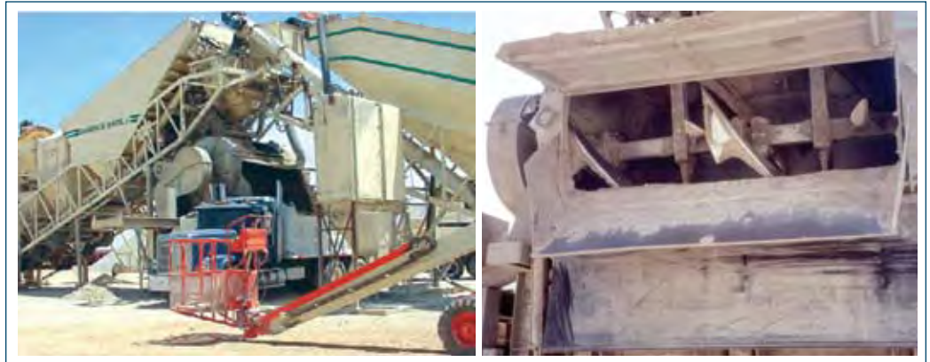
Figure 6-5. Horizontal shaft mixer (left) and close-up view of mixing chamber (right)
