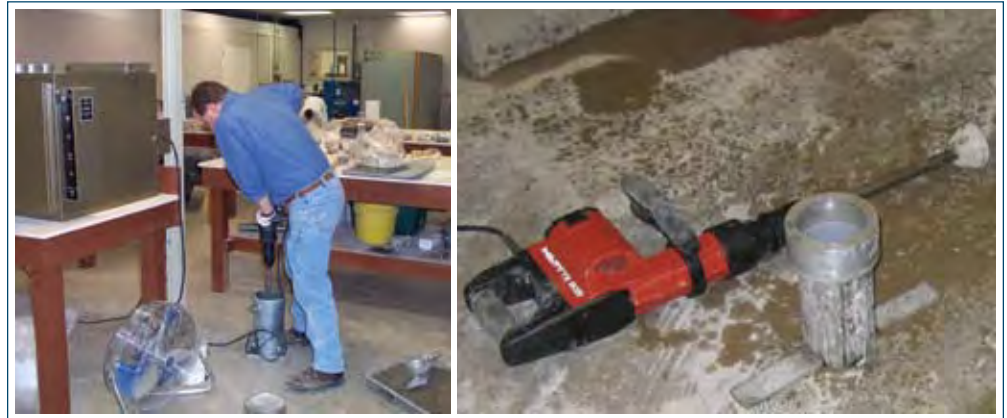
Figure 4-5. Molding RCC cylinder with vibrating hammer
