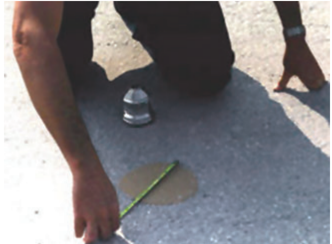
Figure 2.2. Photo of original “sand patch” test using Ottawa silica sand and spreading tool. 14
