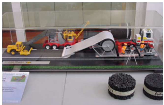
Figure 6.31. Model of "rollable road" surface construction in the Netherlands.
