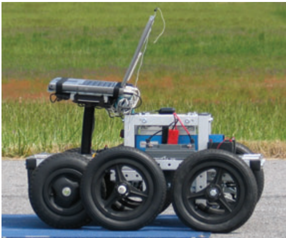
Figure 2.5. Robotic Texture Measurement Device (RoboTex). Photo courtesy of Dr. Robert Otto Rasmussen, P.E., Vice President & Chief Engineer, The Transtec Group, Inc., Austin, TX. 166
