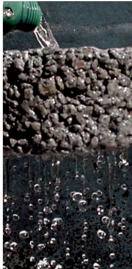
Figure 6.10. Photo of water running through porous concrete. 126
