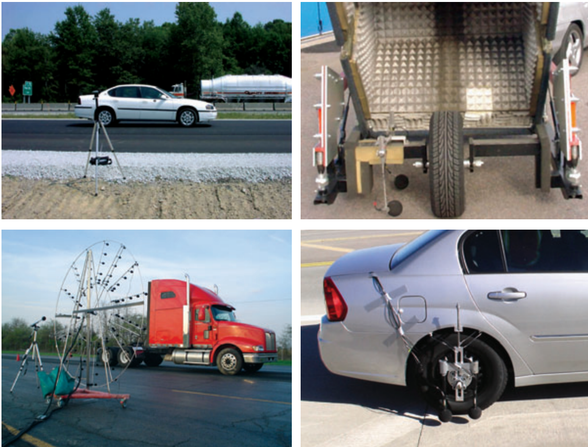
Figure 3.15. Photos of (clockwise from upper left) SPB set-up, CPX trailer, SI equipment and NAH antenna array (courtesy of McDaniel and Bernhard, 163 Ulf Sandberg, Caltrans and Paul Donovan/Caltrans, 162 respectively).
