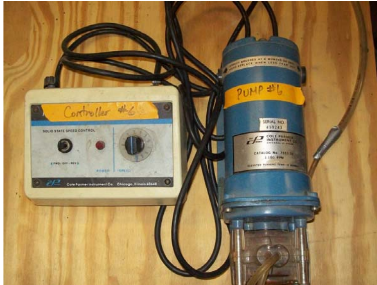
Figure 3.6 - Cole Parmer Masterflex pump
