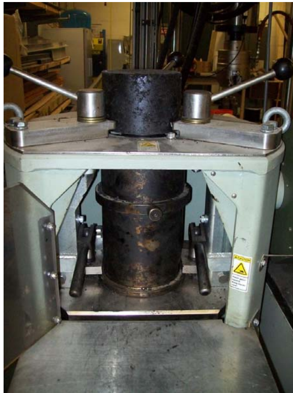
Figure 3.3 - Pine Instrument Gyratory Compactor & Extruded Sample
